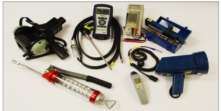
Predictive diagnostic tools utilized throughout MES include ultrasonic tester, combustion gas analyzer, digital volt OHM amperage meter, pulley sheave alignment tool, strobe light, digital thermometer among others.
